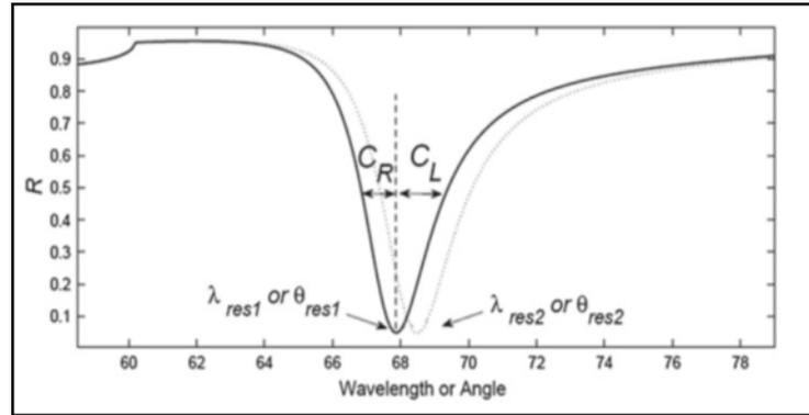
Fig. 3: Surface Plasmon resonance sensor curve [12].
