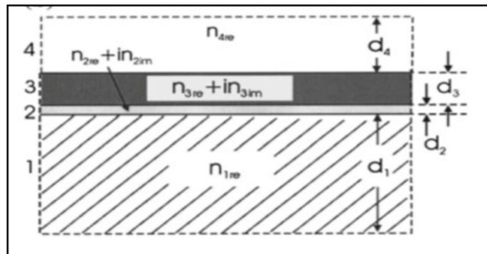
Fig.4: The proposed sensor layers architecture [12].
