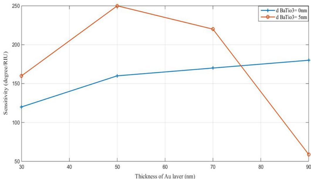
Fig. 6: SPR sensor sensitivity variation against metallic layer Au thickness in BaTiO<sub>3</sub> thickness values (0nm and 5nm).
