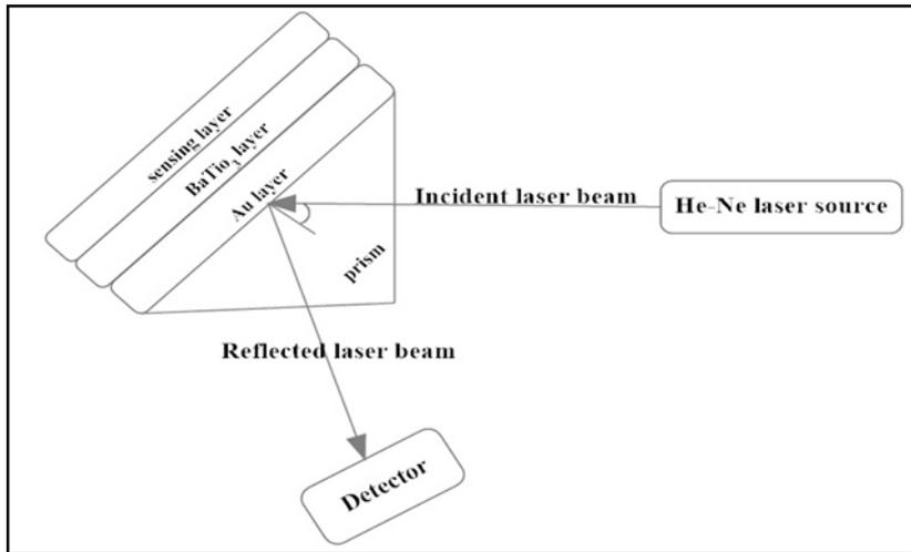
Fig.2: The proposed SPR sensor configuration.
