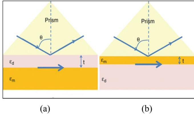
Fig. 1: Surface Plasmon Sensor Configuration (a) Otto type (b) Kretschmann Type
